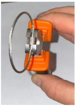
Then press firmly on the crimping tool until the end of the key ring deforms.
